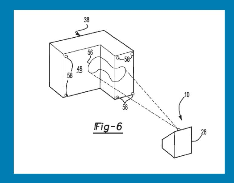
Figure 6 of U.S. Patent No. 10,052,734, at issue in Virtek Vision, depicts the claimed technology: a projector assembly (10) identifying targets (58) on a work piece (38) to project a laser template (56) onto the work piece. The key issue in the case pertained to a motivation to combine references to teach the limitation directed to identifying targets on the work piece "in a three-dimensional coordinate system."
